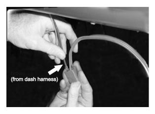
Plug the brown heater feed wire from the dash wiring harness into the open cavity of the heater switch connector, as shown.
