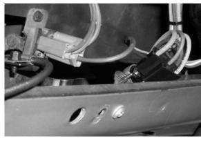
Connect to the heater switch, as shown. Route the remaining 3 position connector to the heater resistor (on top of heater box) and connect.
